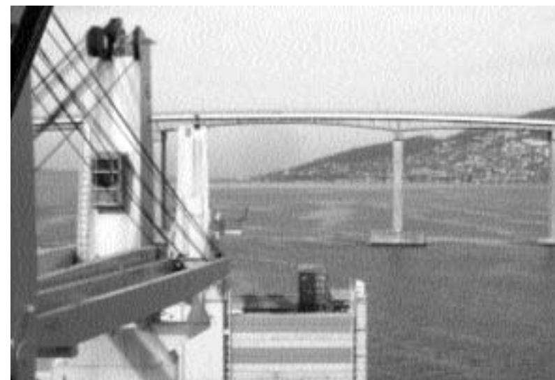
Cape Delfaro 193 x 28 x 10m, approaching Tasman Bridge main navigation span from the north, about 600m off making 9k. The run of the surface current onto the Stb'd 1/4 is apparent looking through the legs to the right, which is why this ship is well over to starboard. From here she drifted across to the centre. A main engine failure at this point is manageable since she has enough way to steer through. Rudder lock is another matter, since the escort tug is only capable of overcoming about 10 deg of helm at 9k. The thing to balance is speed - high in case of engine failure so minimising set and often leeway - and low due to the effective speed of the escort tug. All this is best explored on the simulator.
