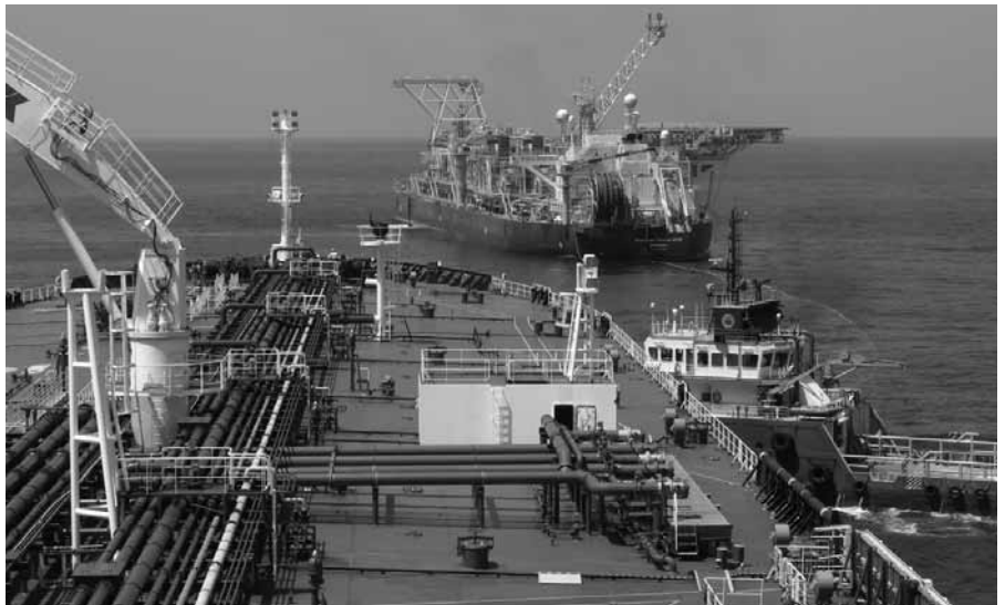
ShuttlePilot is used to line up an offtake tanker with the FPSO Stybarrow on BHP Billiton's Stybarrow oil field off WA
